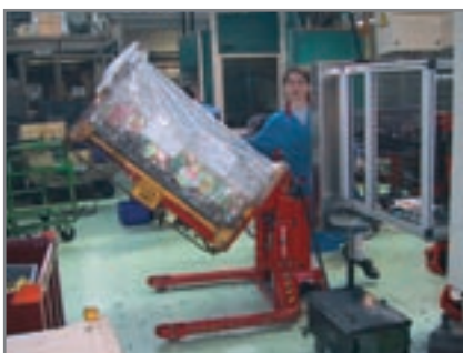
The straddle model makes it possible to handle closed pallets. The Logitilt being used in the component industry.
