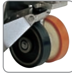
The trucks have at least one vulkollan anti-static wheel in order to conduct away static electricity.
