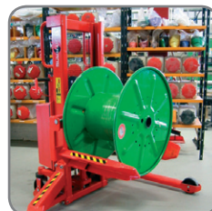
Drum forks when handling barrels.
