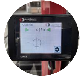
Intuitive screen to preset rotation angles and speed
