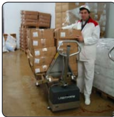
Stainless electric highlifter ensures an ergonomically correct working height in special environments.
