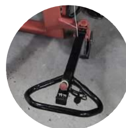
The handle can turn to the side to enable easy operator access
