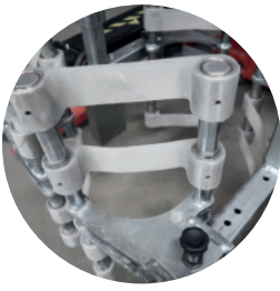
Specially developed polyurethane gripping pads
