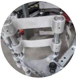
Specially developed polyurethane gripping pads
