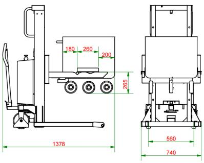
Logitrans semi-stainless steel electric stacker is built with special gripping arms for lifting and handling stainless steel or plastic Eurobin tote bins, with a 200 litre capacity. The arms can be fitted to a **Logitrans straddle stacker**, for lifting and lowering Euro bins. Other lift heights and dimensions are also available.
