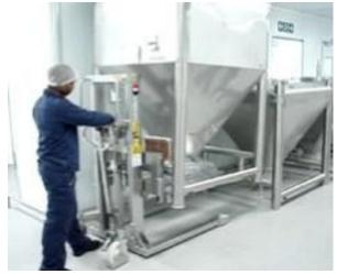
Special fork sizes can also be made for the **Logitrans Rotator**. The IBC can be lifted and turned through 180 degrees each way, so the IBC can **completely emptied** or filled.
