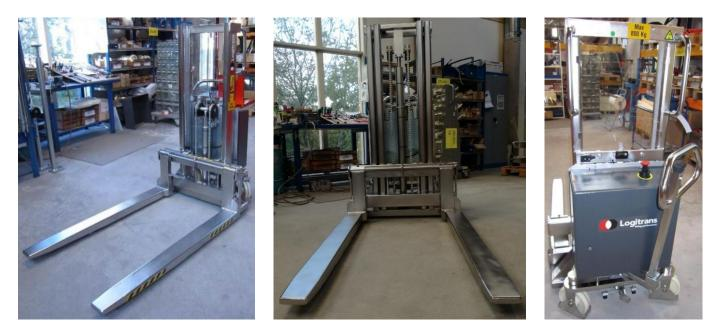
Logitrans EHSS Inox stainless steel electric stacker truck is built with **extra long**, **extra wide** and **extra narrow forks**, for lifting and handling IBCs in a pharmaceutical application.
