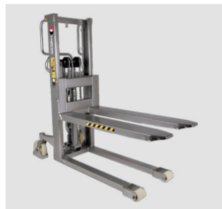
Manual stacker Inox (explosion proof)
