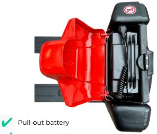
Floating steel battery cartridge
