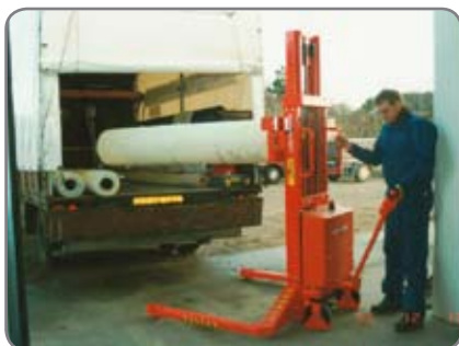
A straddle Logiflex handles reels from a stock to a lorry.
