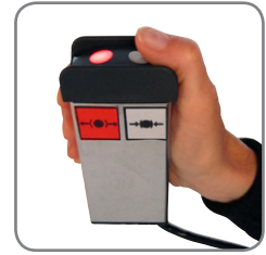
The electric trucks have remote control for reel fastening/releasing.
