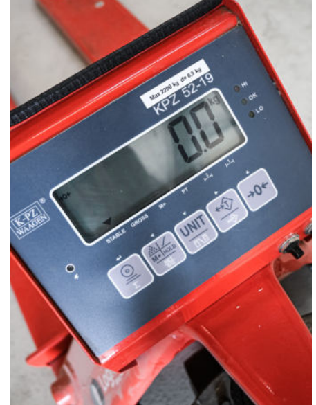
Pallet truck with weighing scale, can weigh up to 2200 kg
