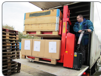
Low own weight means better utilisation of the capacity of the lorry tail-gate.
