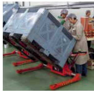
The handle can be turned to the side, so that the user has free access to the contents of the crate or box.
